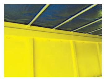
The Open Tops can be supplied with tarps and bows for trans-ocean shipments. Weights and payloads below may change slightly based on whether the units are painted, galvanized or both.
